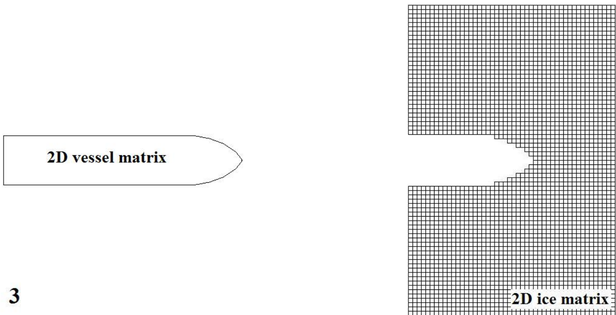
Figure 7.3 The vessel has created a "footprint" in the ice ridge and therefore also in the ice matrix
