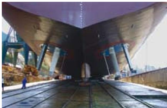
Figure 5: Voith Schneider Propellers fitted on ST216 Edda Fram [4].
