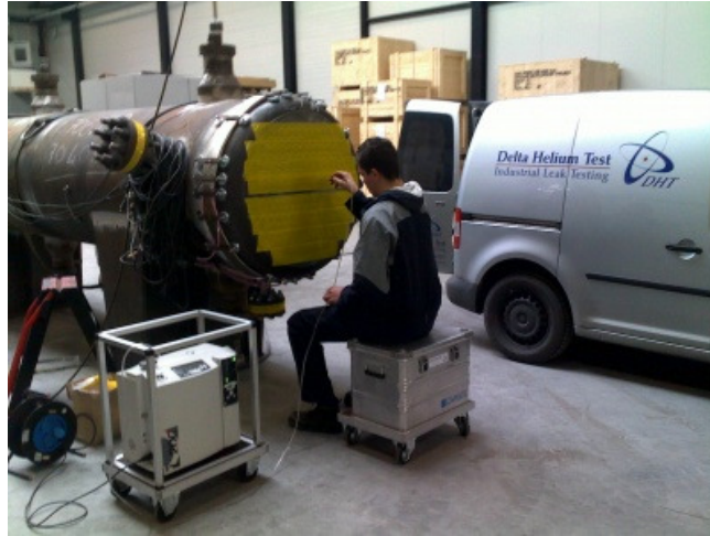
FIGURE 16: HELIUM LEAK TEST (21)
