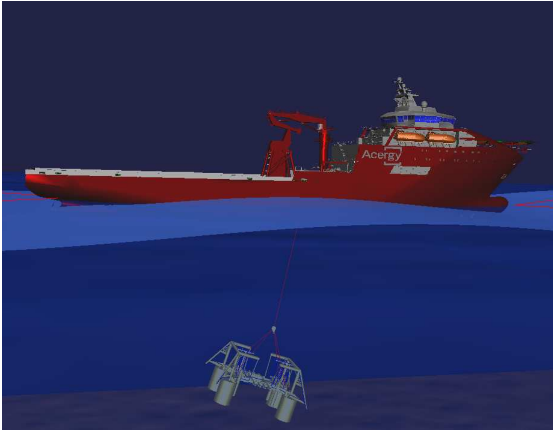
Figure 57 Subsurface towing SIMVIS
