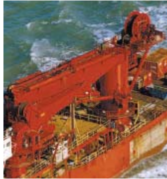
Figure 19 150 tons heave compensated crane onboard Acergy Osprey
