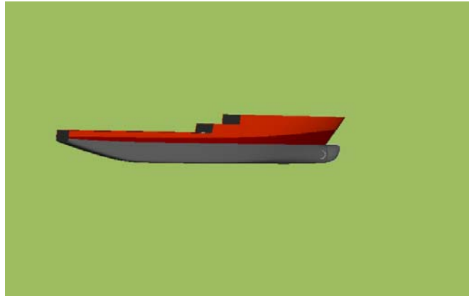
Figure 26 3-D model of the hull with bulbous bow
