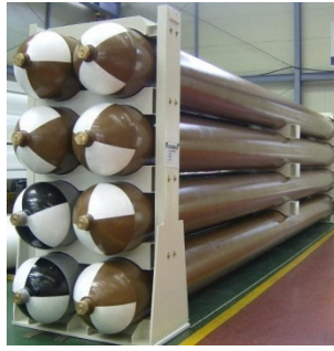
Figure 17 skid mounted gas storage bottles
