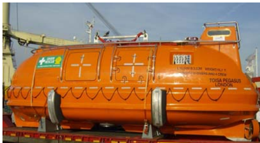
Figure 16 a self propelled hyperbaric lifeboat
