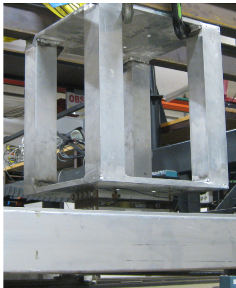
Figure 4.3: Closeup of the force transducer measuring F_{tot}
