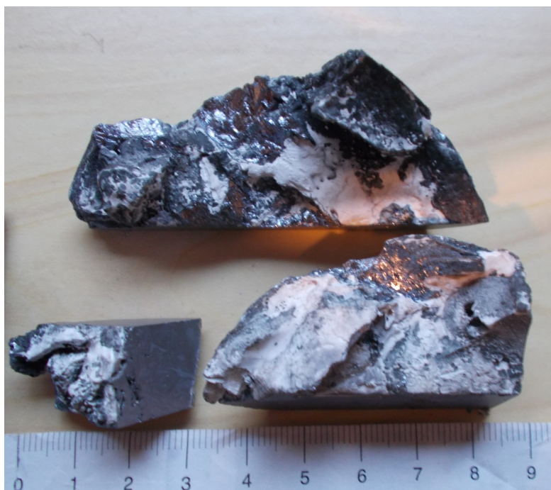
Fig. 70: White layer of oxide covering the top material from the annealed cast at 1200°C for 17 hours
