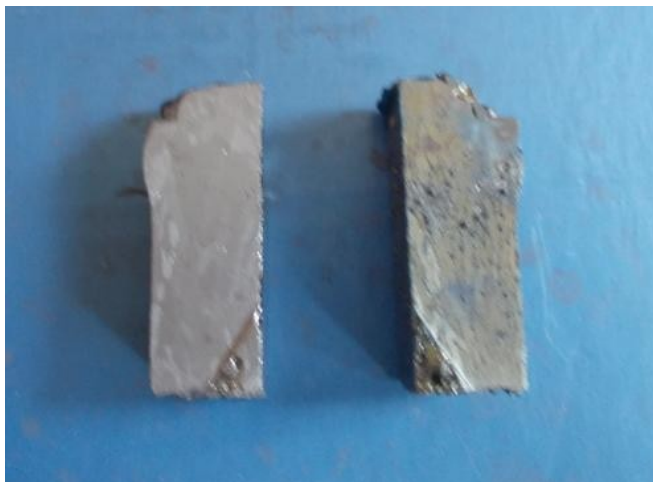
Fig. 35: Sample before (left) and after (right) a heat treatment at 1200°C for 17 hours. The green-blue layer on the surface is made of intermetallic compounds. The same happens for all the samples treated at a temperature over 800°C.
