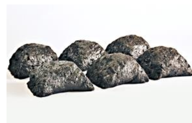
Figure 5 Electrode paste, in the form of briquettes (Elkem)
