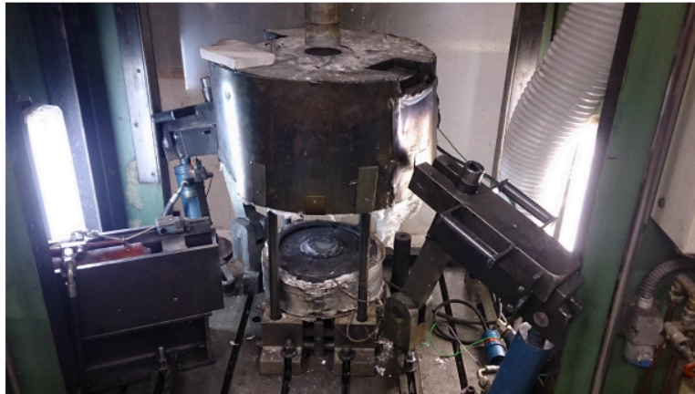
Figure 3.1 Image showing the extrusion press used at SINTEF press laboratory [32].
