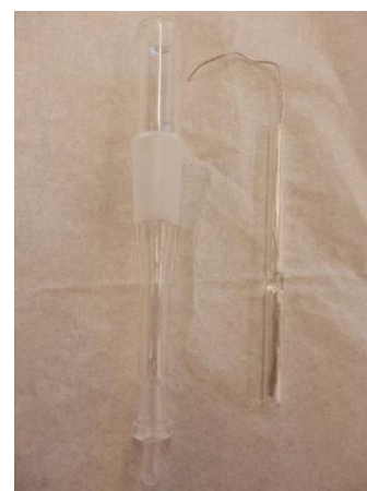
Figure 4-1: Reference electrode. To the right is the tube with platinum wire, and to the left is the outer compartment for this tube.
