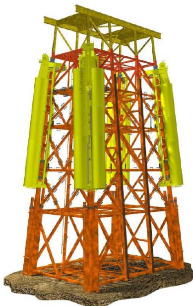
Figure 30: BTA installed at the jacket, (Total E&P Norge AS 2008)
