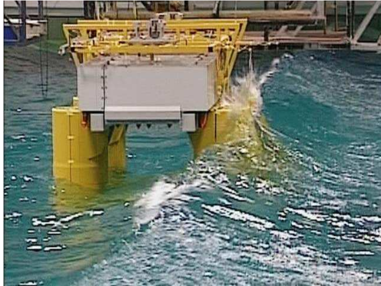
Figure 1.5: Snapshot from a model test for the re-qualification of the Heidrun TLP. Photo: Marintek
