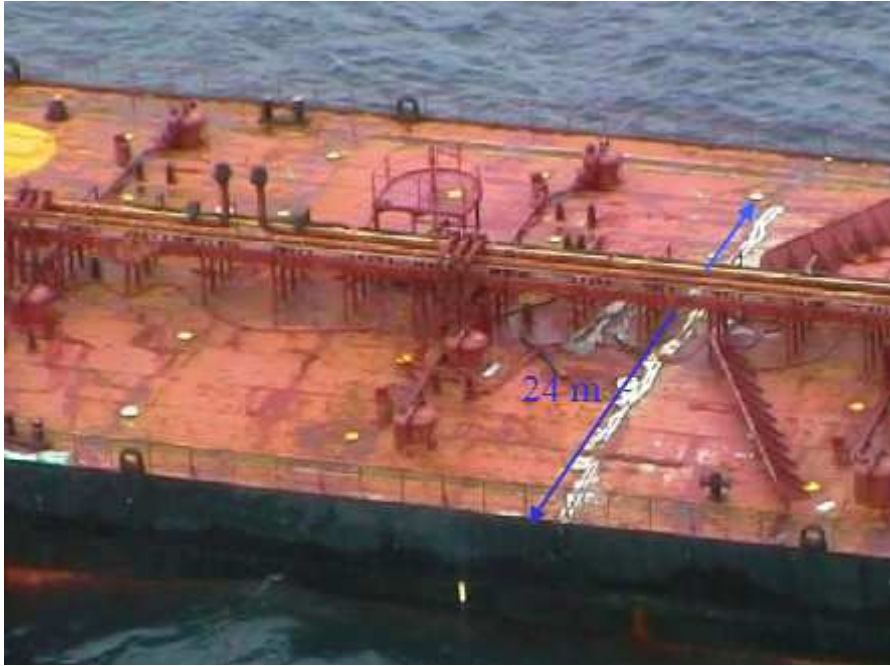
Figure 1.1. Very long crack at deck of tanker Castor, (from ABS, 2001)
