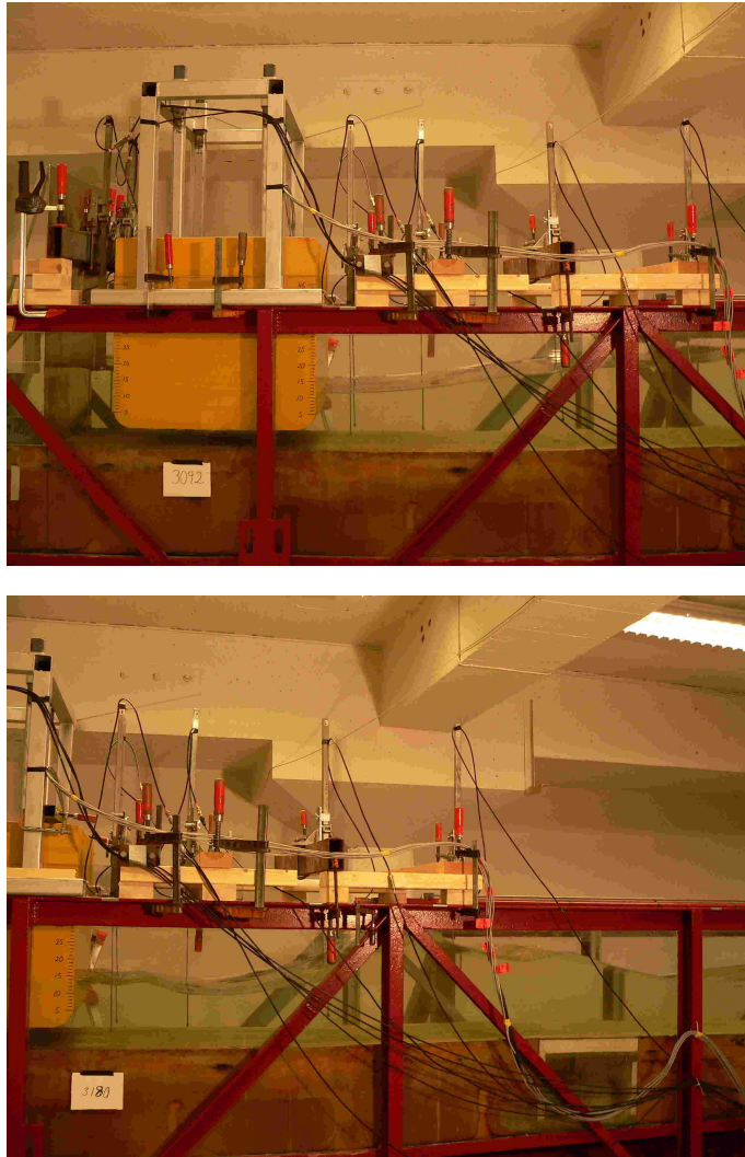
Figure 9.2: Two snapshot from the September 2006 tests. The ship section is fixed and subject to waves entering from the right. The water depth is h = 0.23\text{m} .
