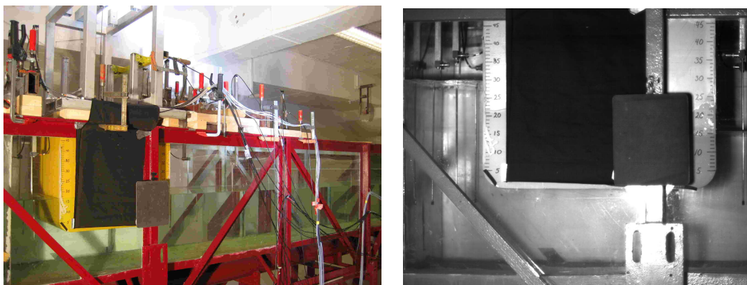
Figure 9.6: November 2006 model tests. Left: Model test set-up. Terminal seen to the far left. Clay and rubber bands were used to seal gap between glass wall and models. The black cloths reduced reflections when acquiring high-speed photos. Right: Sample of high speed camera.
