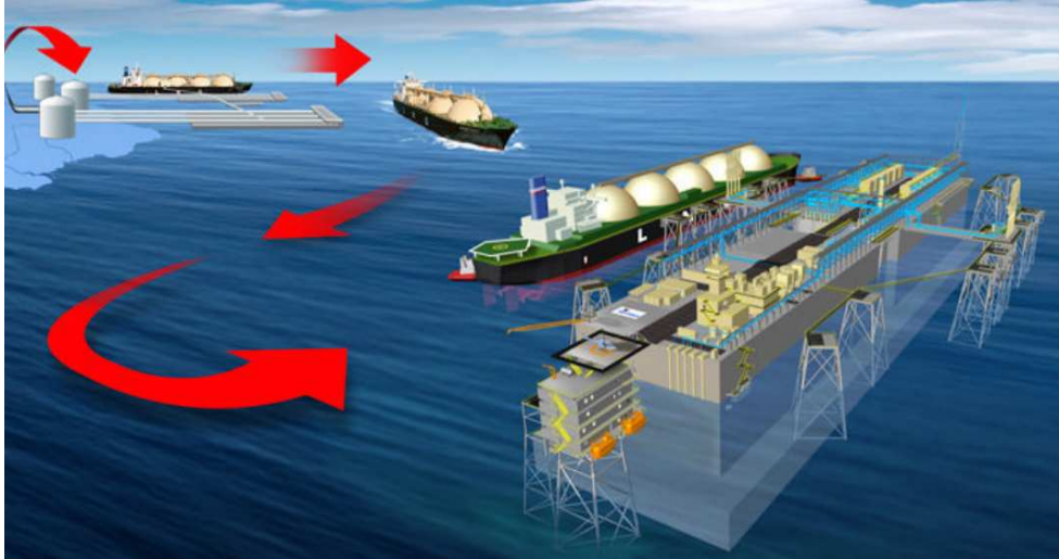
Figure 1.1: Illustration of planned Gravity Based Structure (GBS) type offshore Liquefied Natural Gas (LNG) terminal. Actual site: Port Pelican, coast of Louisiana in Gulf of Mexico (ChevronTexaco). Water depth h = 25\text{m} , distance from land 50\text{km} , GBS dimensions 364\text{m} \times 89\text{m} \times 57\text{m} and storage capacity 330.000\text{m}^3 . The capacity of the LNG carriers is at the present time typically up to 140.000\text{m}^3 and typical dimensions are L \times B \times D = 300\text{m} \times 45\text{m} \times 12\text{m} , where L is length, B the beam and D the draft. The LNG is first off-loaded to the terminal where re-gasified and transported to land by pipelines.
