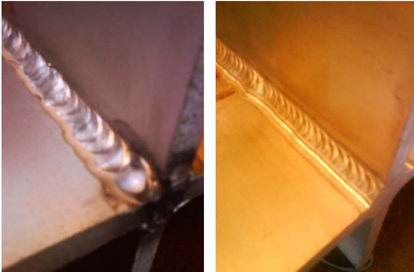
Figure 8-4 Photograph of as-welded (to the left) and toe-ground specimens
