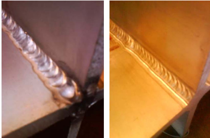
Figure 2-25 Photograph of as-welded (to the left) and toe-ground specimens
