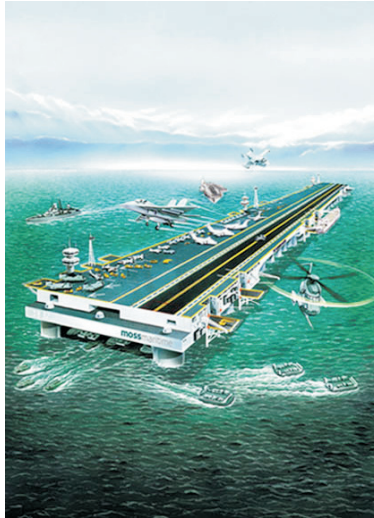
Figure P1.1: Example of interconnected marine structure: floating airport. The illustration is shown by courtesy of Moss Maritime a.s.
