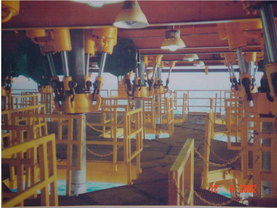
Figure 5.3: Production riser tensioner system at the TLP Joliet (National Oilwell Varco, 2007 b ).
