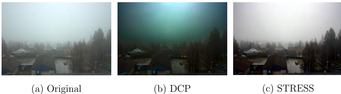
Figure 3.4: Image taken in Gjøvik (Norway) - Lac Mjøsa - at the beginning of the winter 2014-2015. As we can see, the fog on near objects is well removed, far objects still have fog and we do not obtain a saturation effect with (c), that we have in the case of (b).
