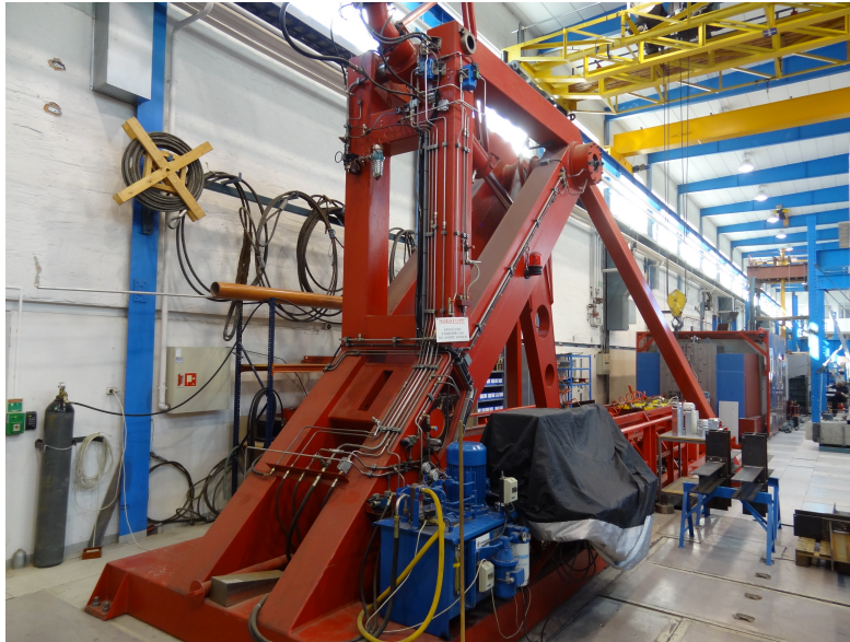
Kicking machine used to accelerate the trolley.
