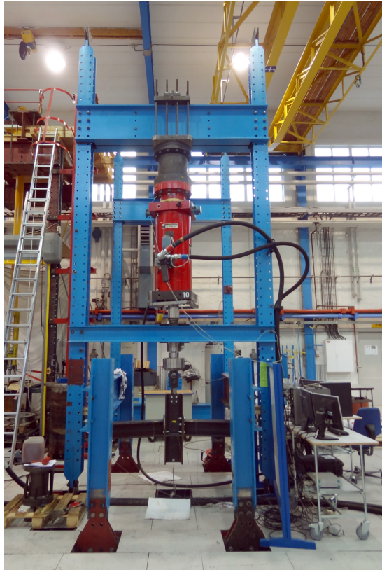
Portal frame structure and the 1000 kN hydraulic actuator
