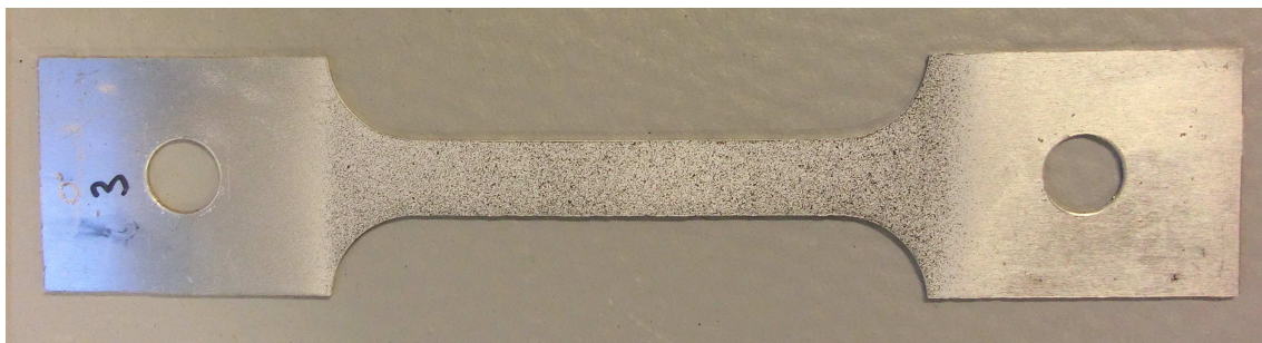
Figure 4.3: Specimen prepared for DIC analysis.
