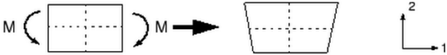
Figure 4.5 Deformation of a linear element with reduced integration subjected to bending moment M.
