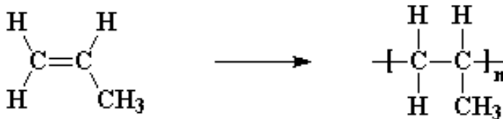
Figure 2.1: Polymerisation of propene to polypropylene
