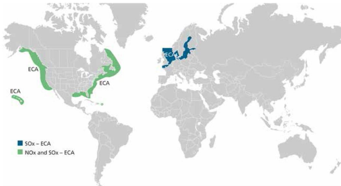
Figure 2-6: Existing ECAs. The sulfur cap applies in all ECAs, whereas the NO x -restriction only applies in ECAs in North America. (DNV GL, 2014a).
