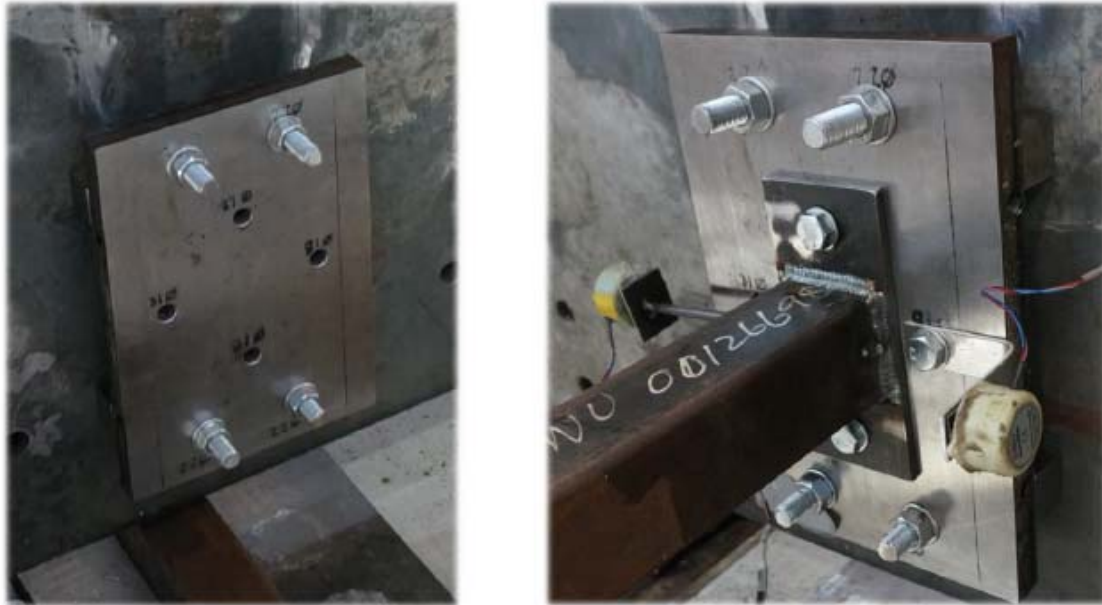
Fig. 4: Support plate on reaction wall (left) and connected Specimen A (right) with rotation gauges.
