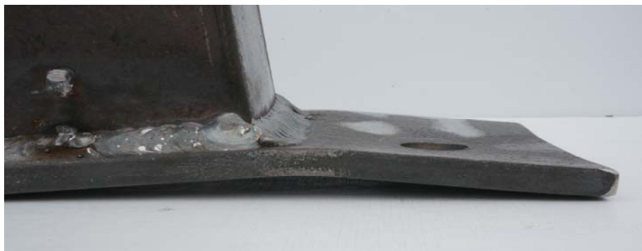
Fig. 7: Deformed end plate of Specimen A, close-up of extending part at tension side.
