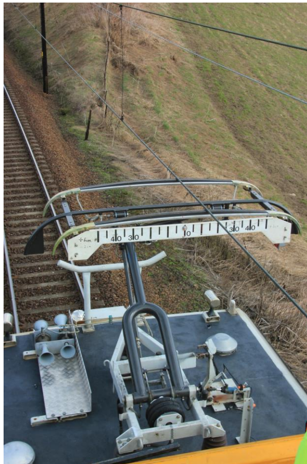
Figure 21 How the contact wire slides on top of the pantograph.
