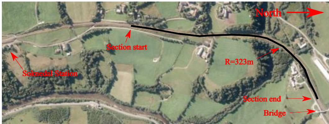
Figure 11 The geometry of the studied railway section seen from above. The black line marks the track. The figure is based on [10].
