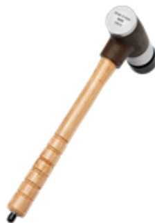
Figure 38 Modal hammer, Brül and Kjær type 8208[51]
