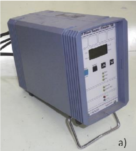
Figure 40 Signal conditioner/power supply, Kistler Type 5134[52]
