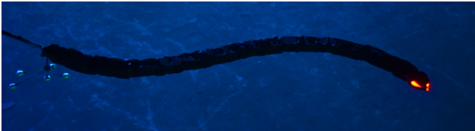
Figure 5.15: The underwater snake robot Mamba in the pool at MC-lab with the markers attached to the tail for position measurements.
