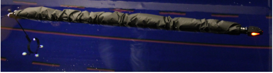
Figure 6.26: The underwater snake robot Mamba in the pool at SINTEF flume tank with the markers attached on the tail for position measurements.
