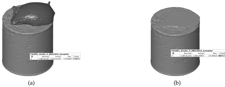
Figure 6: Large excessive mass located at the bottom of FA20D1 sample 4. Figure a) shows the excessive mass marked, and in b) the mass is removed and the hole sealed.
