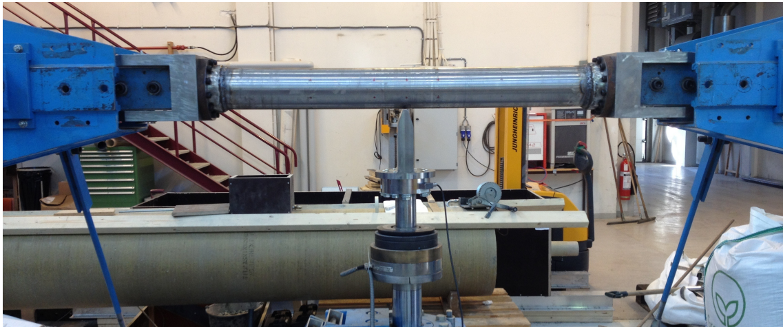
Figure 6.6: Pipe 1 mounted in the stretch bending rig prior to testing.
