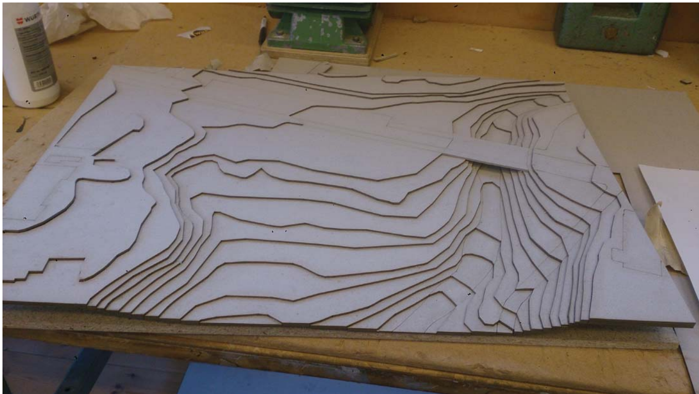
Prepared file for cutting. Lasercut. Glued the pieces together.
