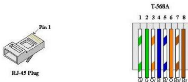
Figur 3.5: Fargekode for kobling i RJ45 plugg [7]
