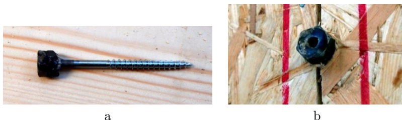
Figure 4.13: Screws for Attaching Accelerometers
