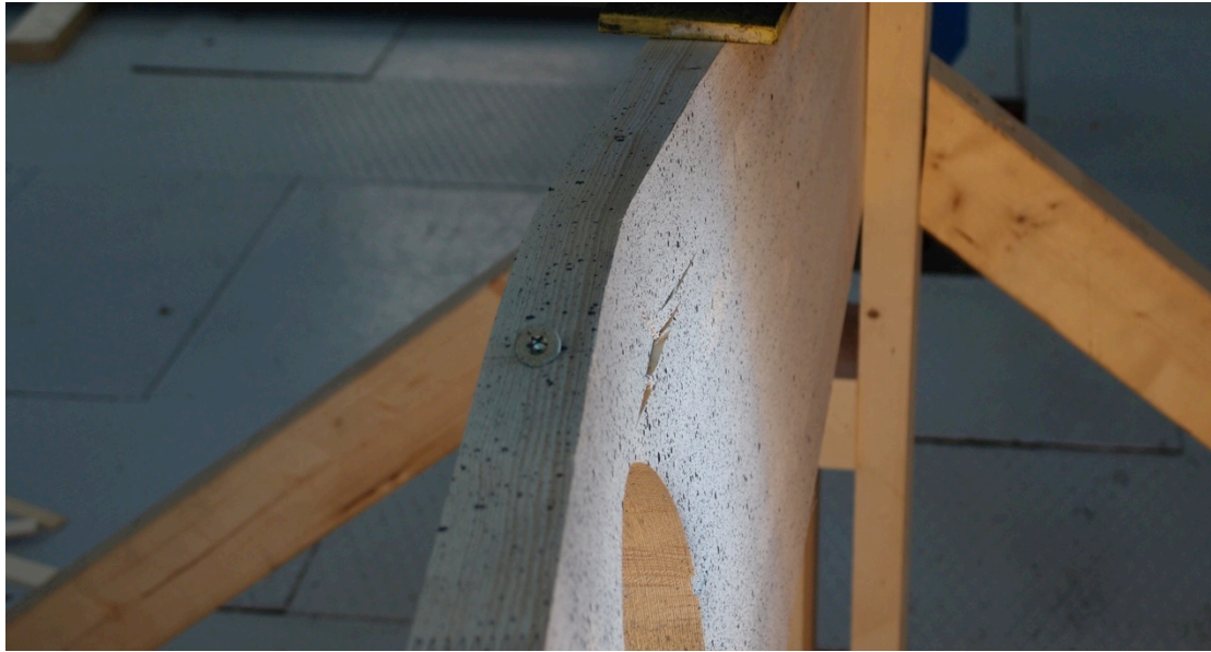
Figur 144: Stage 500, Utbøyning + sprekk
