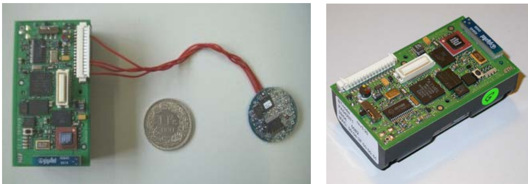
Figure 17. BTnodeRFID reader, and the same reader compactly packed [56]
