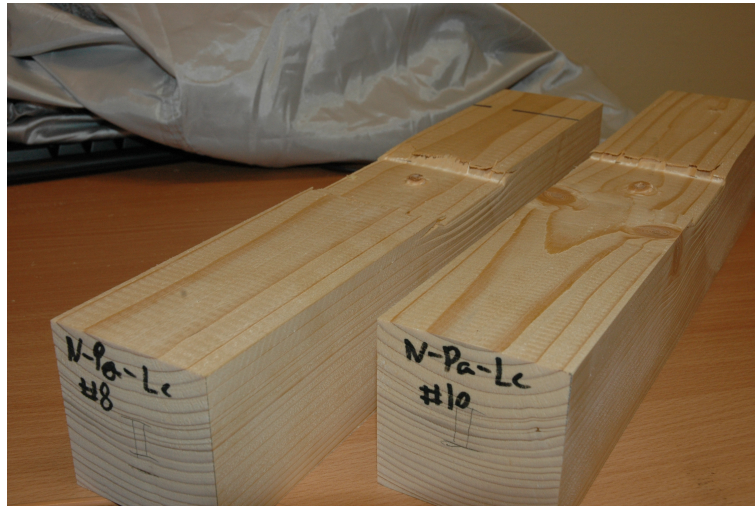
Figure 4.7: Knots in specimens 8 and 10
