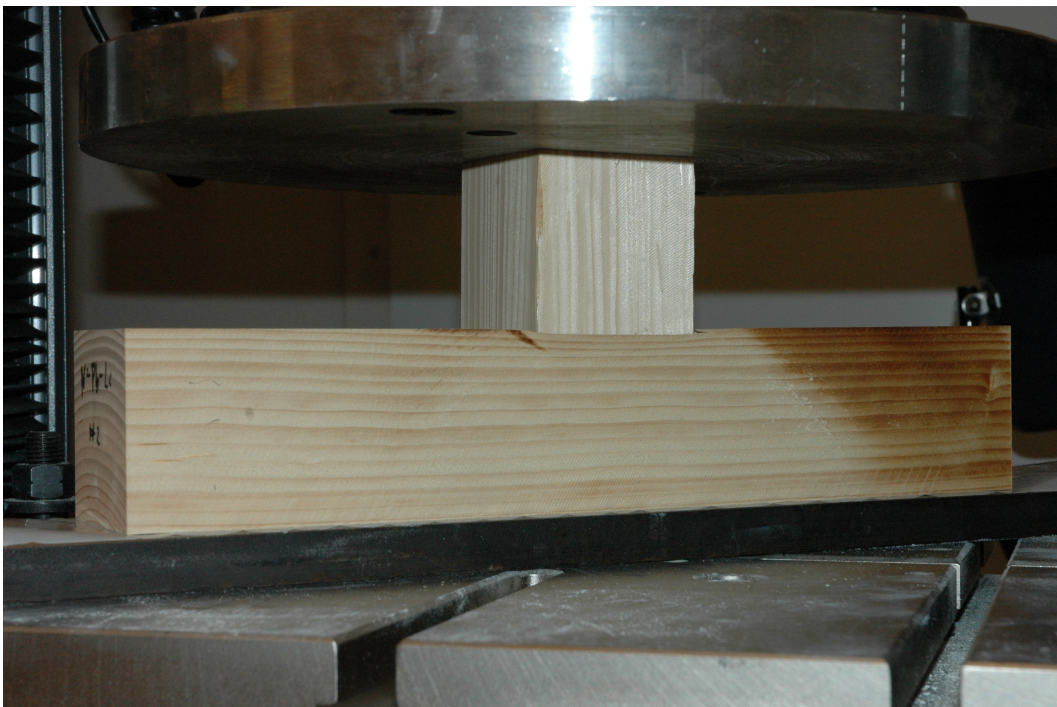
Figure 4.2: Sill being compressed in the testing machine
