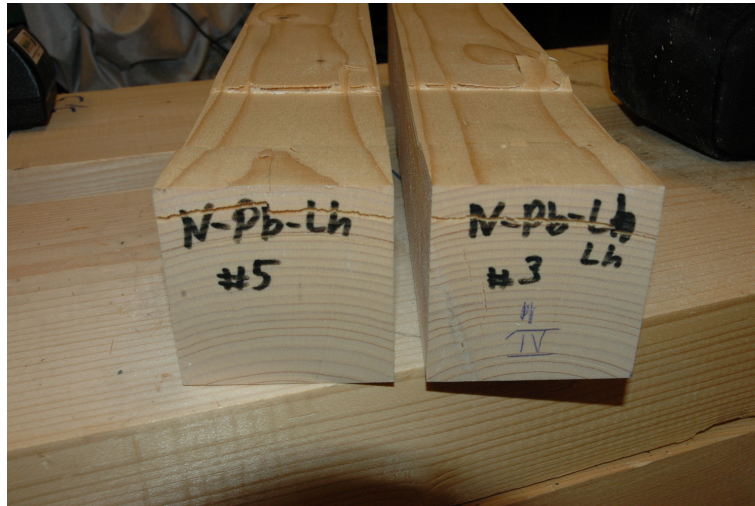
Figure 4.9: Examples of horizontal cracks reaching the edge of specimens
