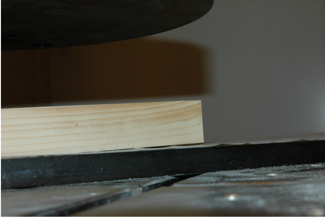
Figure 6.1: Lifting of the ends of a H-Pb-Lc sill
