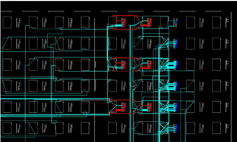
Figure 5.4: Example of a completed rerouting process with only legal wires
