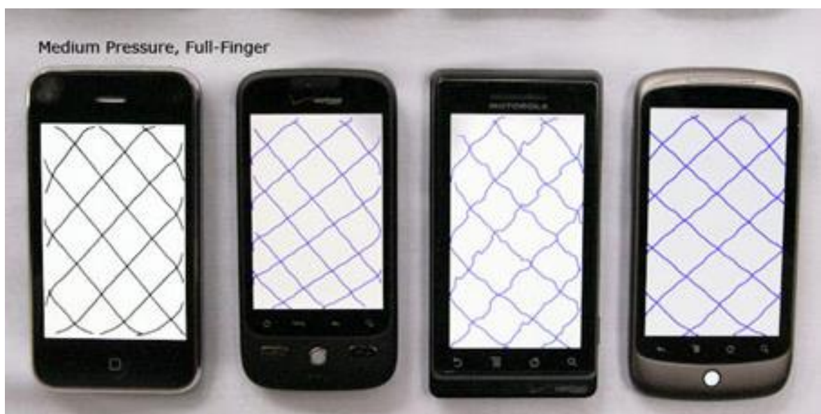
Figure 1.5: Comparison of signal processing capabilities on mutual capacitance touch screens [7]
