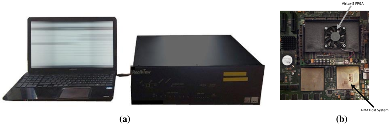
Figure 2.10: (a) The SHMAC set-up in the current thesis, (b) snapshot of the interior part of the RealView Versatile platform
