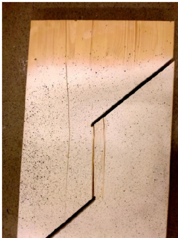
**Figure 38: Cracks forming from top of specimen**
