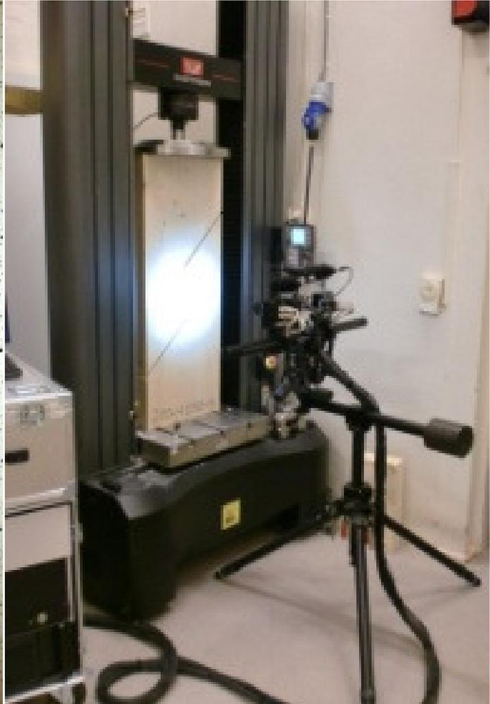
**Figure 10: Specimen in INSTRON test machine with cameras and spotlights on tripod fixed at the area of interest**
