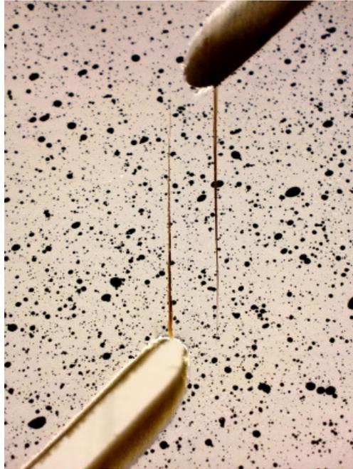
**Figure 20: Two vertical cracks forming between cuts**
