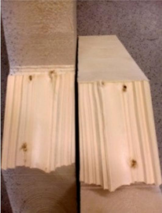
**Figure 26: Specimen split in half at failure forming one shear plane**
