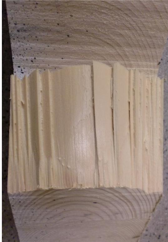
**Figure 46: The shear area after fracture change between tracing the annual rings tangential and “jumping” from rings in radial direction.**
