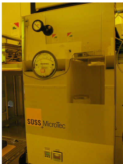
Figure A.1: SUSS SCIL subassembly. Dial near top controls imprint pressure. Gauge in the middle shows imprint pressure. Displays near bottom show pressure (left) and vacuum (right).
