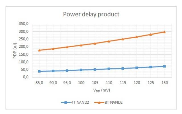
Figure 7.13: The power delay product in the ring oscillators constructed of 4T and 8T NAND2 gates.  $V_{DD}$  was increased from 85mV to 130mV.
