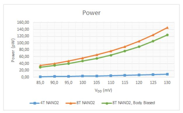
Figure 7.31: The power consumption in the ring oscillators constructed of the NAND2 gates.  $V_{DD}$  was increased from 85mV to 130mV.
