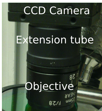
Figure 3.1: The 'camera' consisting of an objective, 20 mm extension tube and CCD camera.
