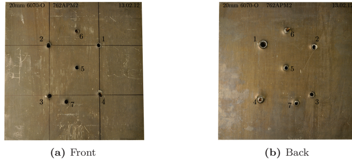
Figure 4.4: Impacted AA6070-O plates.
