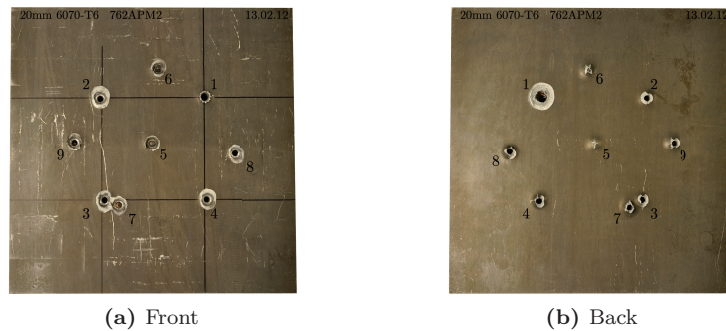
Figure 4.8: Impacted AA6070-T6 aluminium plates.
