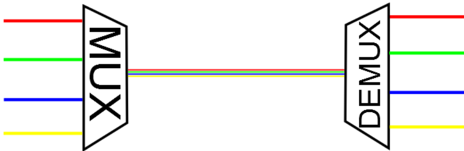
Figure 3.7: Operating principle of WDM. Each color represents a different wavelength. The different wavelengths are combined onto single fiber by a multiplexer and then demultiplexed onto four new fibers.
