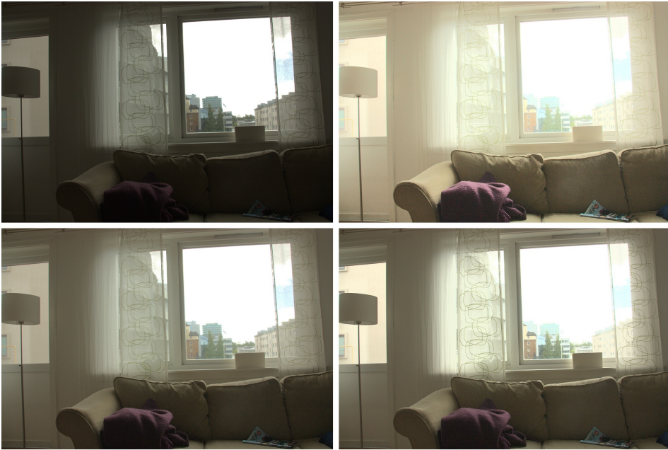
Figure 50: Top left, alpha 0 (linear mapping equal to original). Top right, alpha 1 (histogram equalization). Lower left, alpha 0.5. Lower right, reduced histogram curve.
