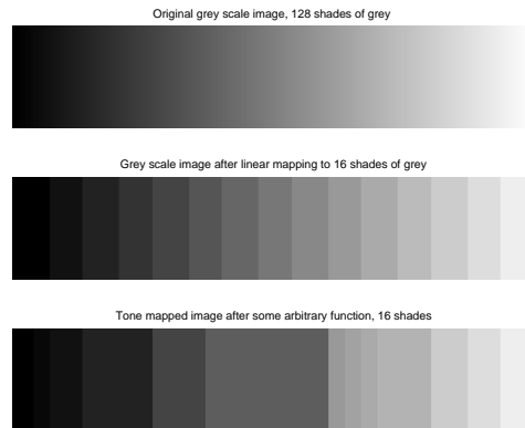
Figure 15: Figure showing how a gray scale image will be tone mapped in two different ways. Original image on top. Shades goes from 0 to 127 with one column of black pixels at end to limit the image. In the middle, the scale from the first are simply linearly transformed. This means that all the new values cover the same number of old values. The bottom part of the figure show tone mapping with an arbitrary operator. Here the new values does not cover the same amount of old values. In this particular example, more weight are given to one of the shades in the middle.
