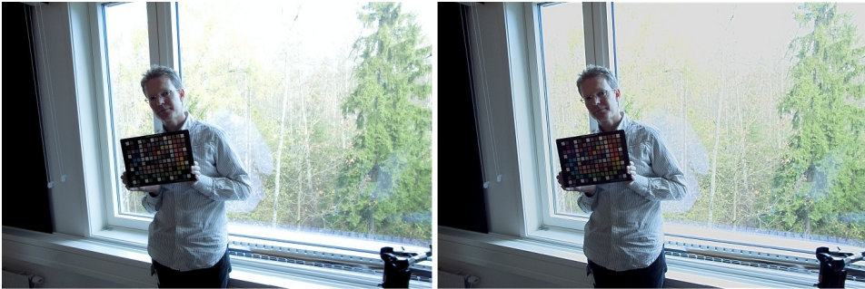
Figure 63: Left image is tone mapped with Duan and Qius algorithm with alpha 1. Right image is tone mapped with Reinhardt's photographic tone mapper.
