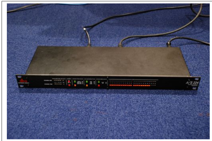
Figure 4.4: The DBX AFS224 connected to the system loop.
