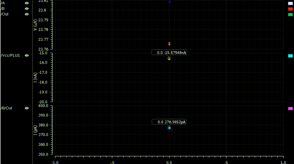
Figure A.5: Static Power Consumption, NOR Design (A=0, B=0, Y=0)
