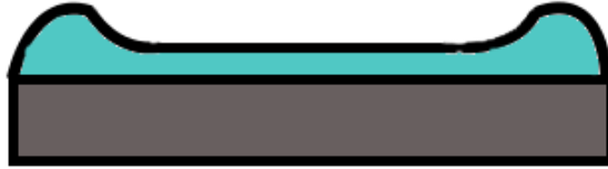
Figure 3.1: Illustration of the edge bead effect, exaggerated for illustration purposes. The blue area represents resist on top of silicon.
