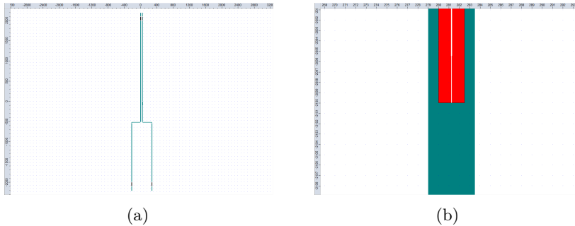
Figure 4.6: The fourth mask design, including inverse tapered waveguides for external coupling. Consists of one reference waveguide and a waveguide with resonators. This mask is given slight changes throughout this work.
