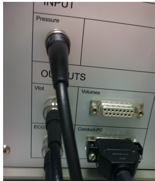
Figure 44: Leycom Sigma 5DF. Takes pressure as input to show PV-plots on another screen. Volume is generated by the unit and is available through an output channel. ECG is also available.
