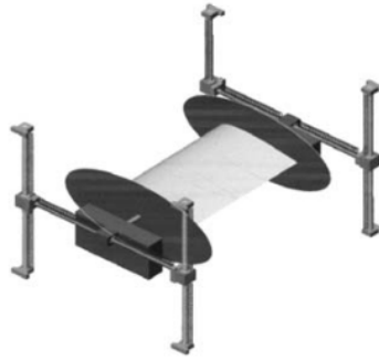
Figure 1.2: Rig allowing three degrees of freedom [10,37].
