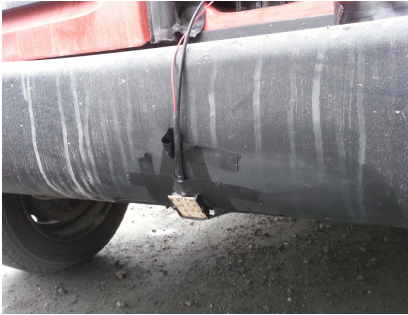
(a) Close-up photo of the radar sensor mounted on the rear bumper
